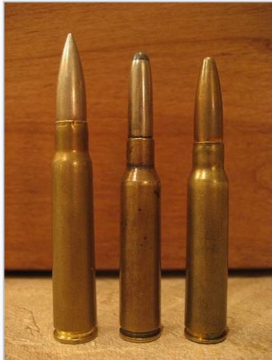
(Left to Right) 7.92mm Mauser (also called 8mm Mauser), 6.5mm Carcano, and 7.35mm Carcano
